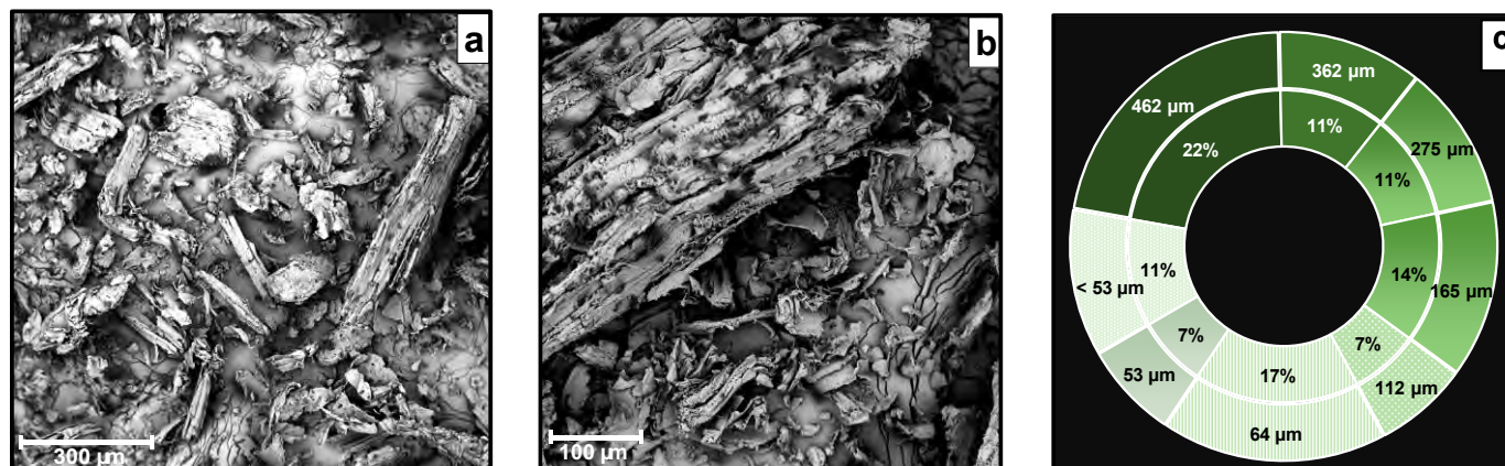
Figure 1. Topinambur residue characterization, scanning electron (SEM) micrographs at (a) 250× (b) 530× and (c) particle size distribution.
